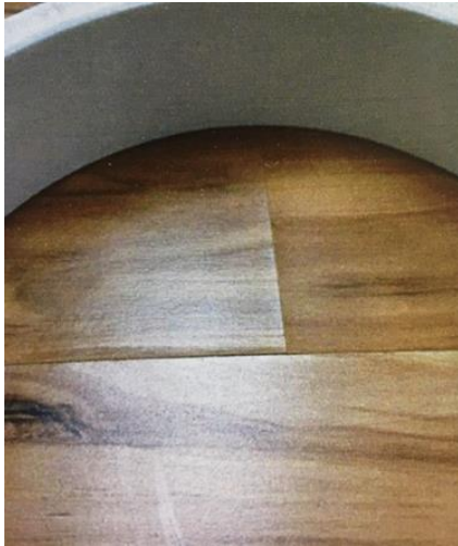
Level 3: failed test (Source: NALFA)
